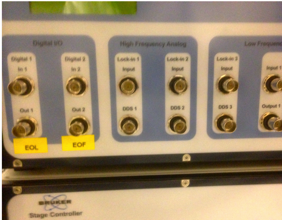
Fig. 6: The EOL and EOF triggers are on the front of the NS-V controller. Make the connections as labeled in the image.
